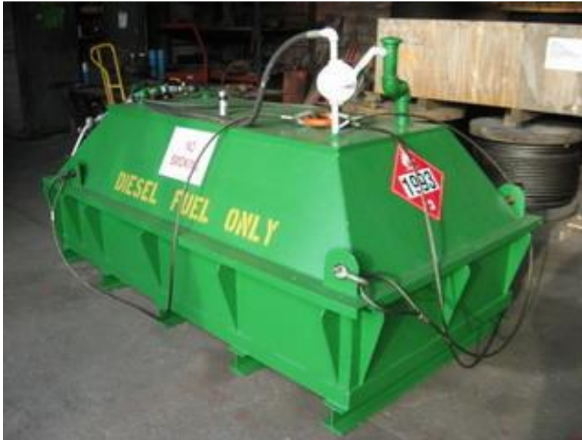
Figure 15-1. Portable tanks for fueling crane
